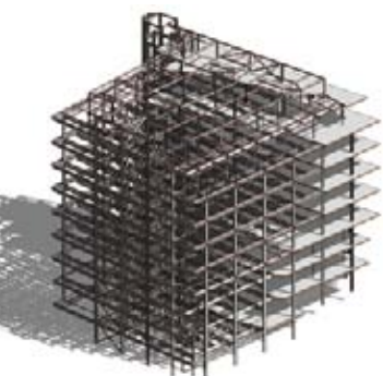
Below right: Long 10.5m spans are a feature of all floors.
